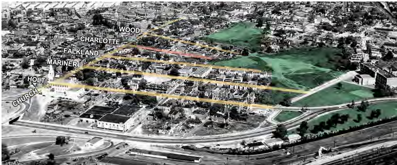
Figure 4-5: Mid-Century aerial photo of Tidewater Gardens area prior to demolition with colors added to illustrate the extent of greenspace where the creek was filled, high streets (yellow) and the low Charlotte Street alignment. (NRHA)
